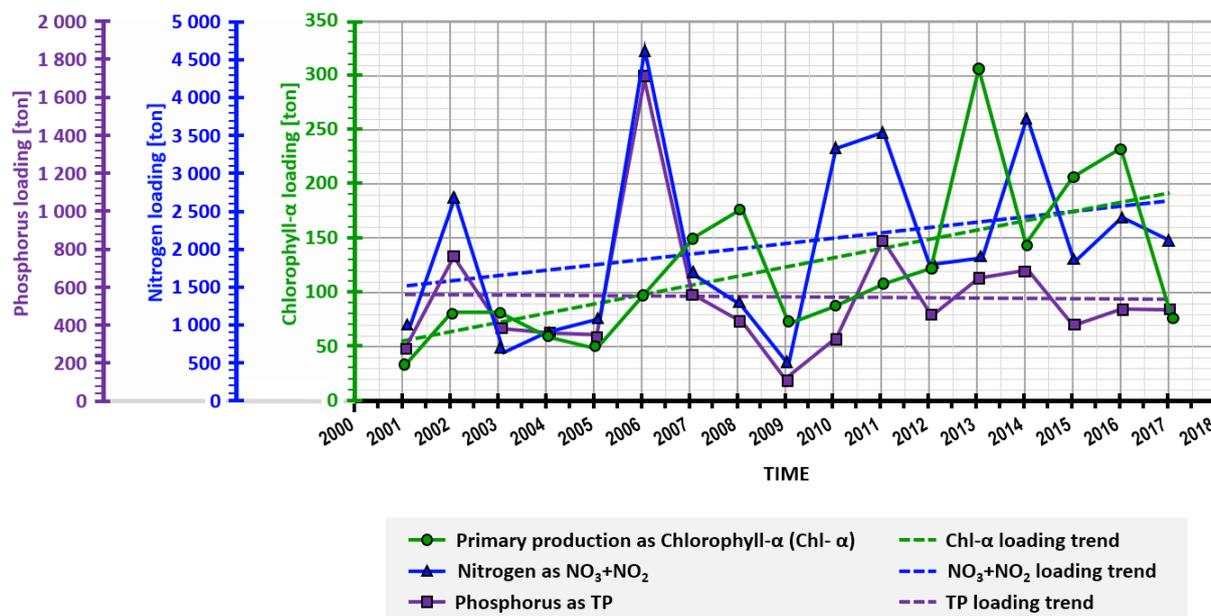
**FIGURE 4: Annual phosphorus and nitrogen-loading of, and primary production in six large South African dams.**
